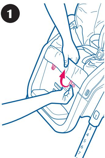
Remove the seat pad by unfastening elastic straps from bottom of seat, shown.
